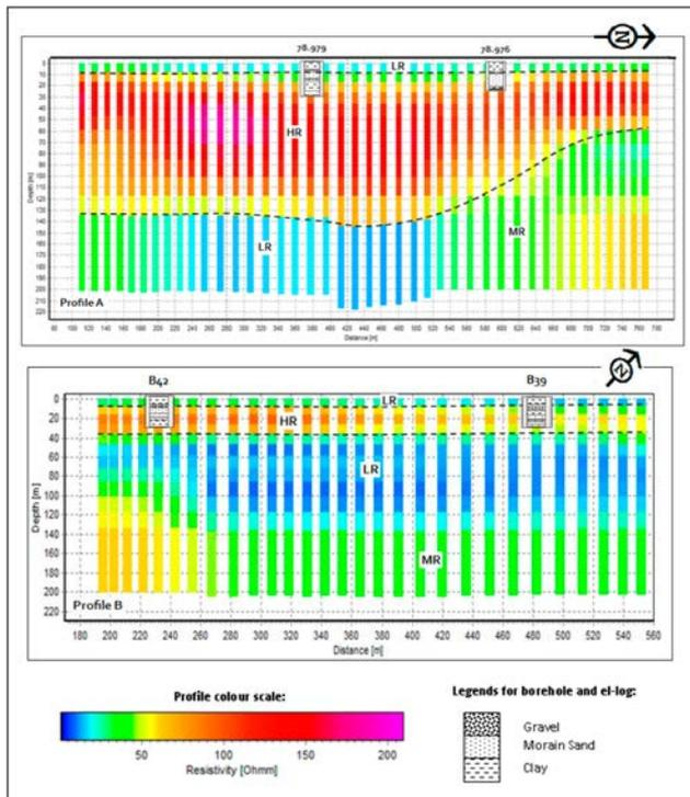
**Figure 9:** Vertical profile shows the layer that possibly contains the buried valley. Profile A and B are profiles on the southern and northern portion of the survey area respectively. HR, MR and LR stand for high, moderate and low-moderate resistivity.
