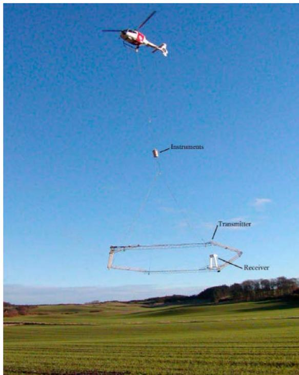
**Figure 5:** SkyTEM in operation (courtesy of SkyTEM Aps).
