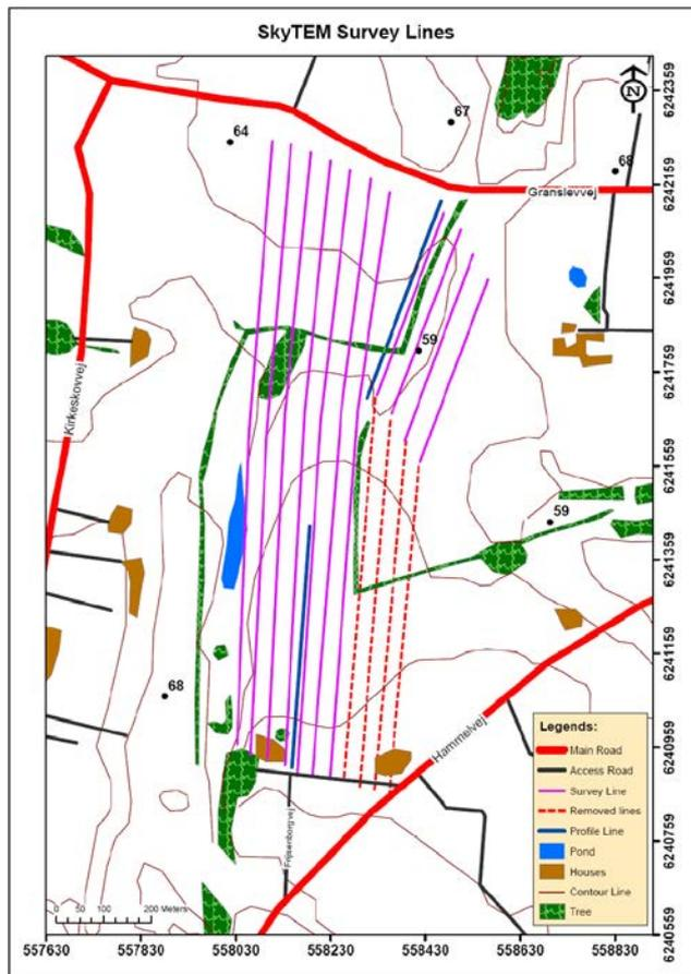
Figure 6: SkyTEM survey lines.
