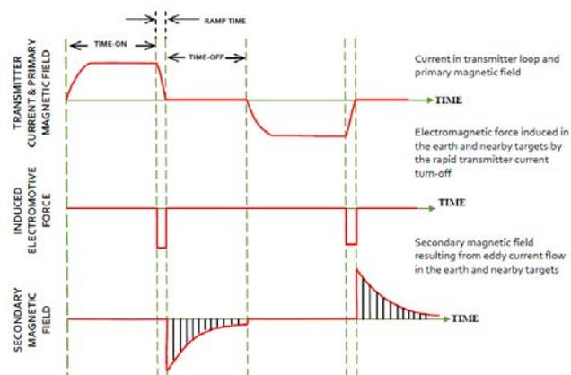
**Figure 3:** TEM (Transient Electromagnetic) waveforms (after McNeill, 1990).
