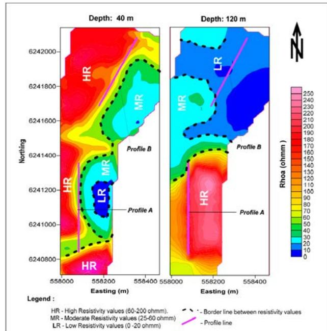
Figure 7: Average resistivities in selected intervals. It shows two different interval resistivity maps which is for 40 m and 120 m depth. Purple lines are the line of selected sounding point that used to plot the vertical profile (Figure 9). Coordinate system: Euref89 zone 32N.
