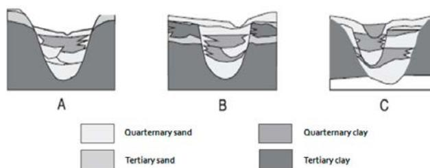
**Figure 2:** Sketches of possible types of buried valley erode into clay dominated sediments (after Sandersen *et al.*, 2003).
