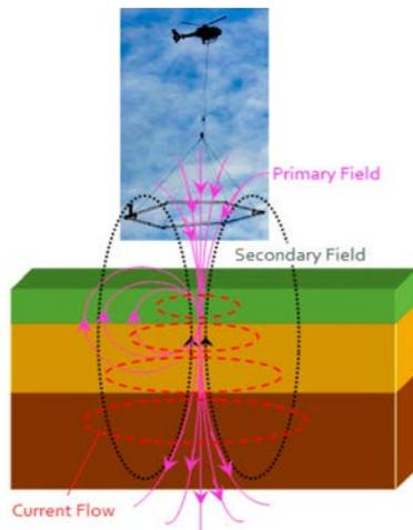
**Figure 4:** TEM (Transient Electromagnetic) eddy current flow.
