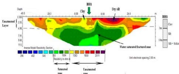
Figure 2: Resistivity image at BH1 (electrode spacing 2 m).
