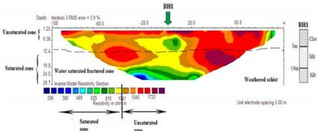
Figure 3: Resistivity image at BH1 (electrode spacing 5 m).
