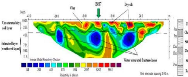
Figure 4: Resistivity image at BH7 (electrode spacing 2 m).
