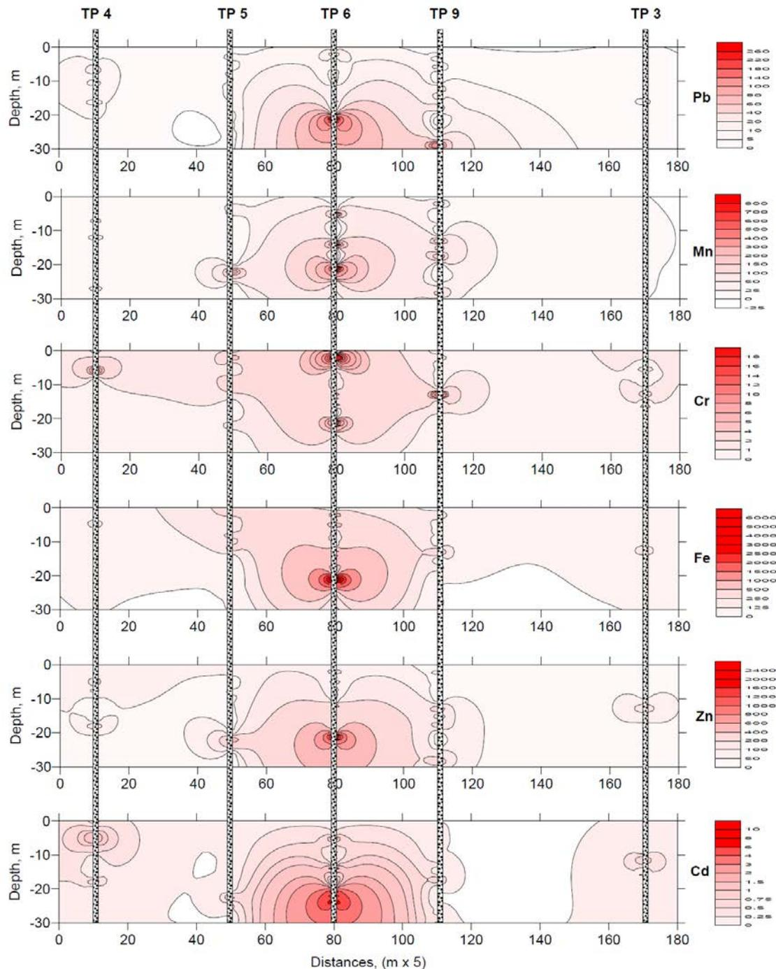
**Figure 3:** Contour diagrams of heavy metals distribution profile at boreholes TP4- TP5-TP6-TP9-TP3.
