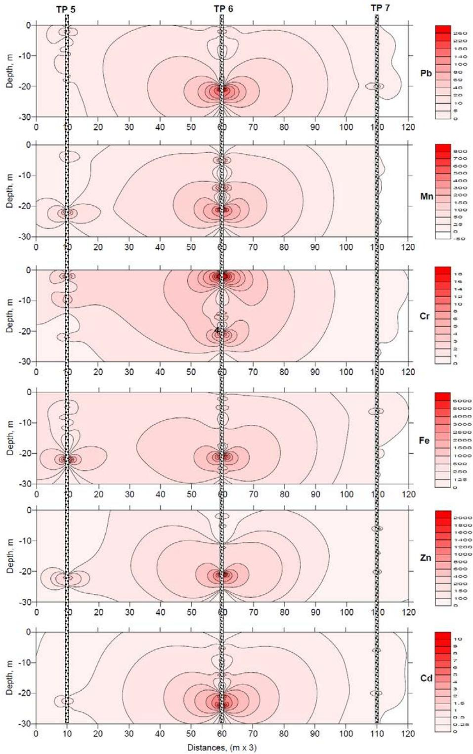
Figure 4: Contour diagrams of heavy metals profile at boreholes TP5-TP6-TP7.
