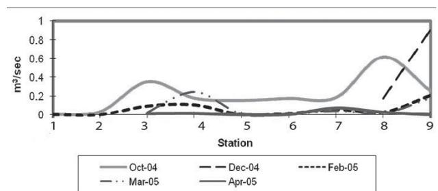
**Figure 8:** Stream flow distribution in 9 sampling stations.
