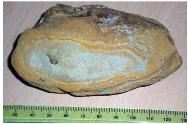
Figure 2: Concretionary layers (yellow colors being dominant) encompassing a Fe-depleted mudstone from another facies. Note the sharp boundary between both materials.
