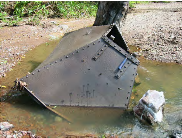
Figure 8: Remains of a side-tipping wagon used to transport manganese ore boulders to the wharf at Tanjung Batu, Marudu Bay
