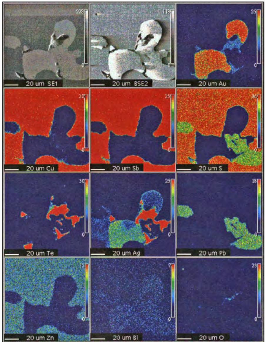
**Figure 4:** Electron Probe Microprobe Analysis (EPMA) of Ajmal Mine gold ore. Note the presence of Au and Ag of native gold, Te-Ag-Au in petzite. Native gold is associated with tetrahedrite (Cu-Sb-S) and galena (Pb-S).
