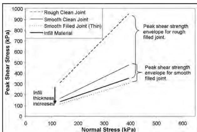
Figure 9: Peak shear strength envelope of various types of joint.
