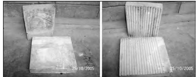
**Figure 4:** Cast joint blocks; smooth (planar) and saw-toothed (rough) surface.
