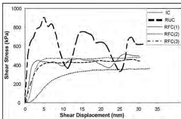
Figure 8: Shear stress-displacement curves for rough joint (clean and filled), under normal stress C = 396 kPa.
