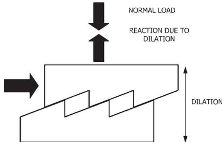
**Figure 2:** Fluctuations of normal stress due to dilation.
