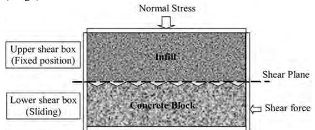
**Figure 5:** Test setup for direct shearing of the infill on rough joint surface.
