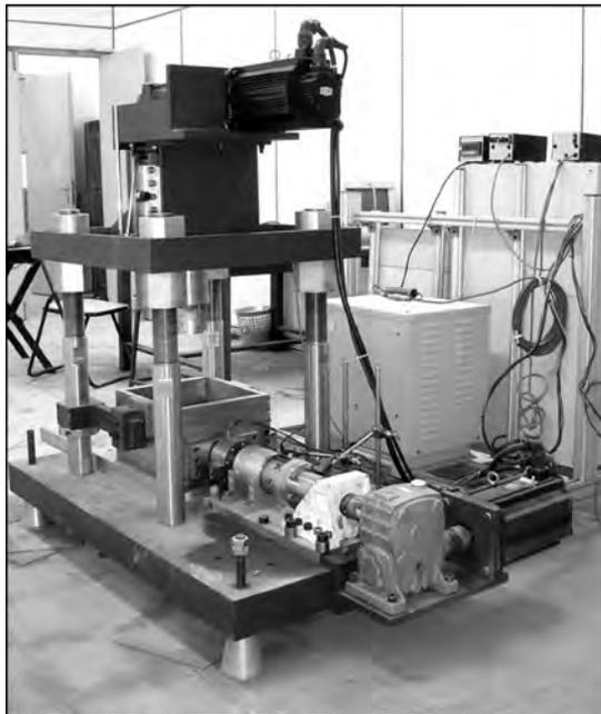
**Figure 3:** Servo-controlled direct shear test equipment.
