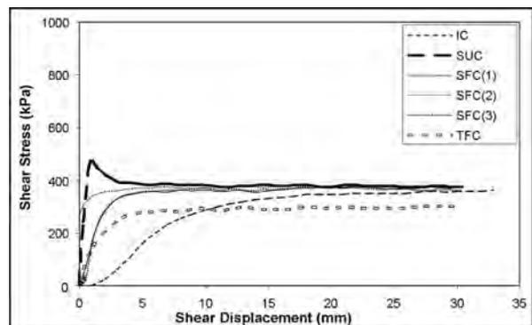
**Figure 7:** Shear stress-displacement curves for smooth joint (clean and filled), under normal stress C = 396 kPa.
