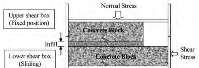
**Figure 6:** Test setup for shear test on filled joint (sandwich shear test).
