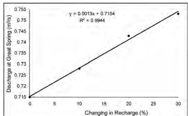
**Figure 14:** Sensitivity analysis of recharge.
