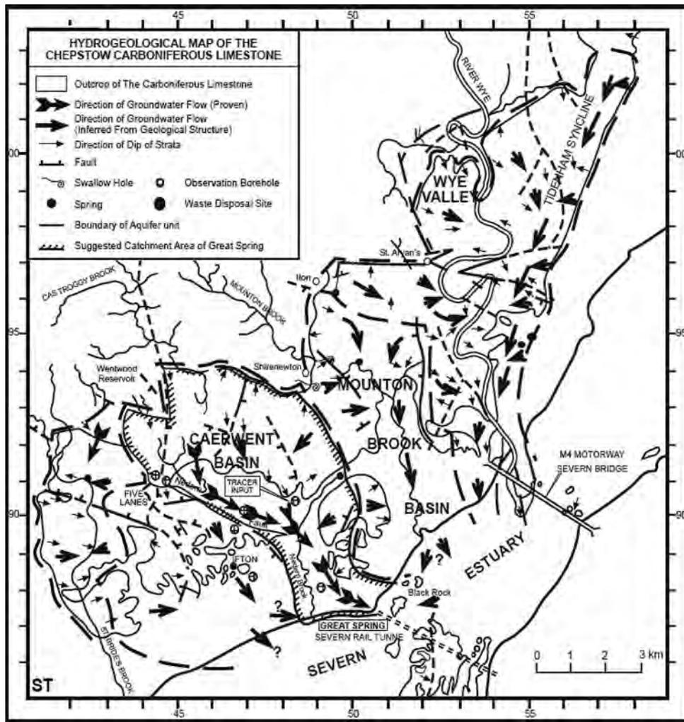
Figure 2: Hydrogeological map of Chepstow Block Carboniferous limestone.
