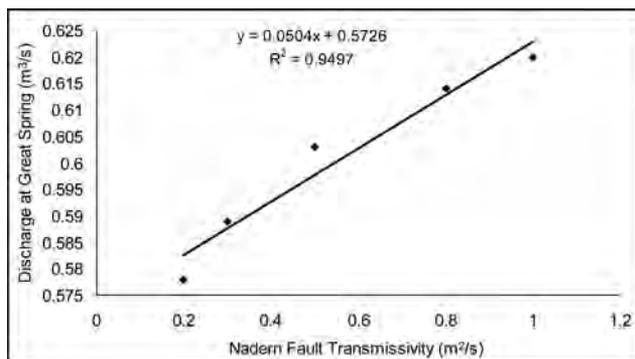
**Figure 13:** Sensitivity analysis of the Nadern Fault.
