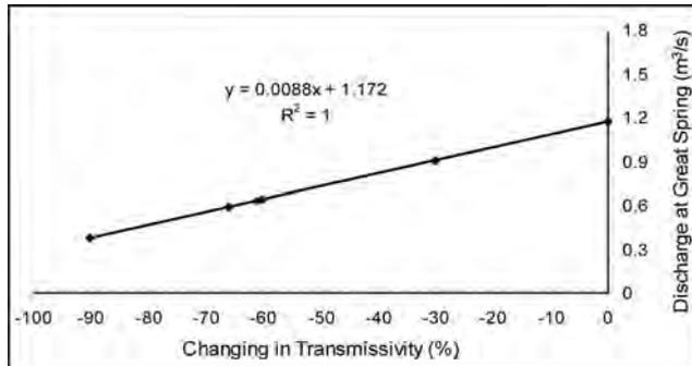
**Figure 11:** Regional transmissivity – Great Spring discharge sensitivity analysis.
