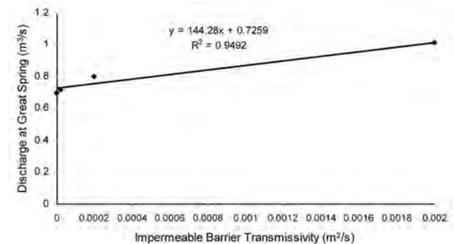
**Figure 12:** Sensitivity analysis of impermeable boundary.
