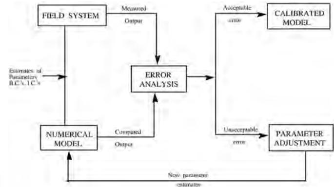
Figure 6: Trial-and-error calibration procedure (modified from Anderson & Woessner, 1992).
