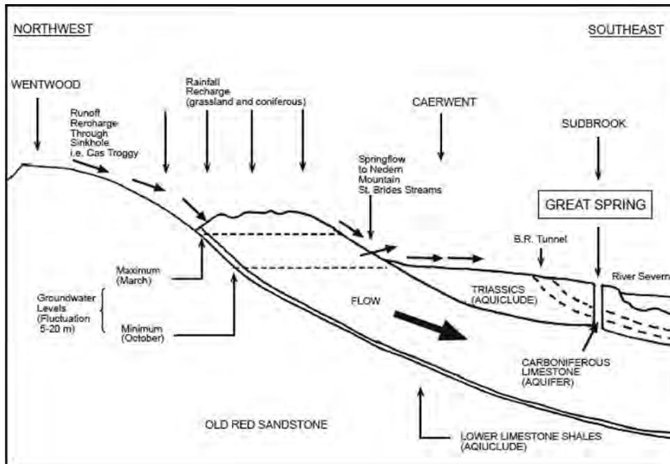
Figure 3: Hydrogeological cross section of the Carboniferous limestone aquifer from Northwest to Southeast.
