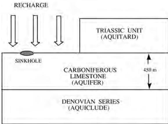
Figure 4: Conceptual model of the Chepstow Block limestone aquifer.
