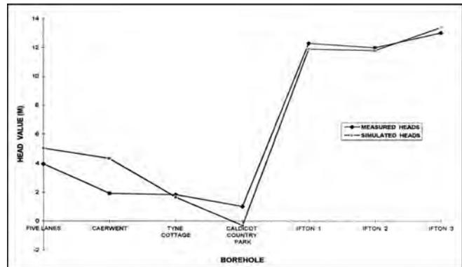
Figure 10: Comparison of measured and simulated heads.
