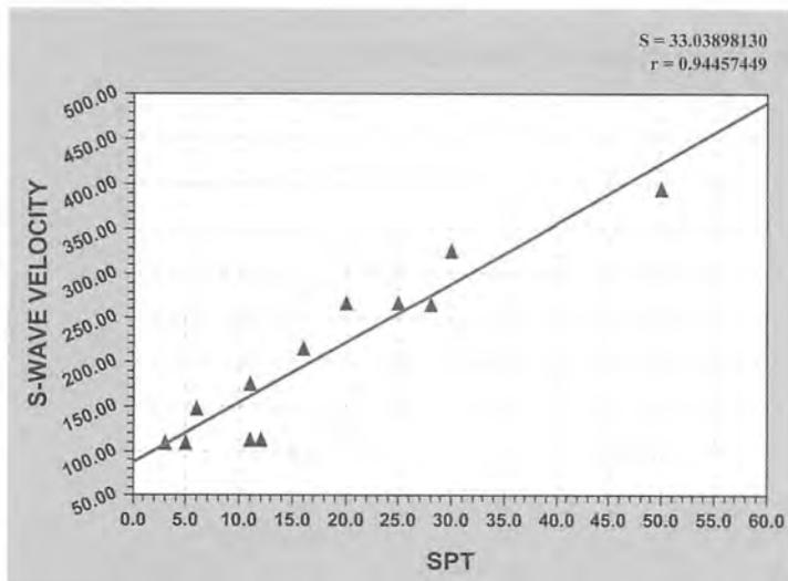
**Figure 8:** S-wave versus SPT plot
