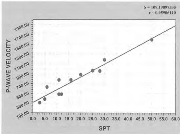
**Figure 7:** P-wave versus SPT plot
