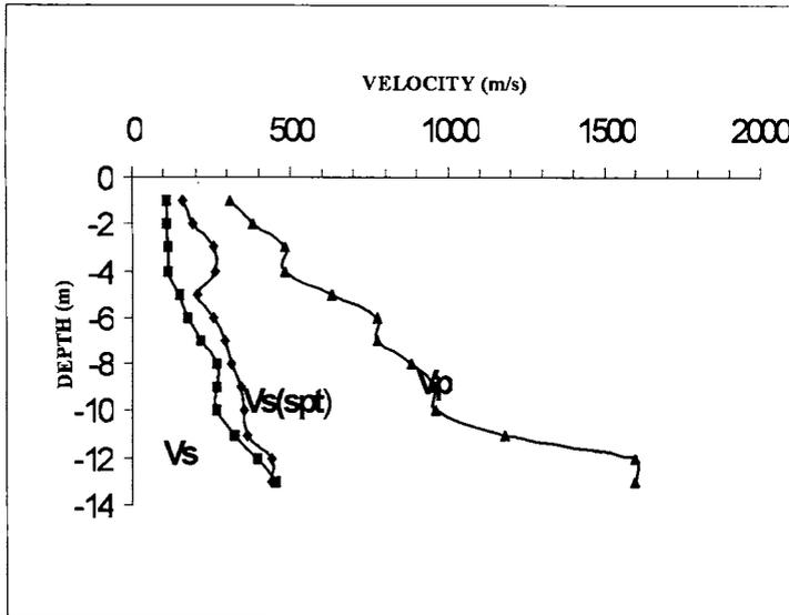
Figure 6: P-S waves curves versus depth
