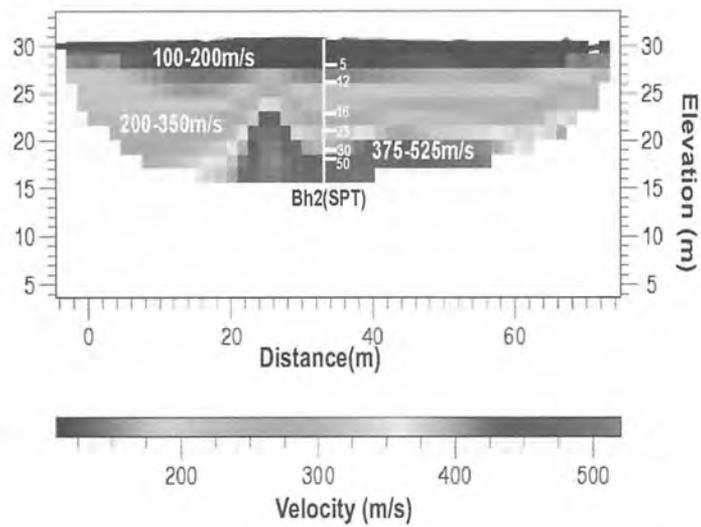
**Figure 4 (top):** P-wave velocity model of a survey line near borehole 15
