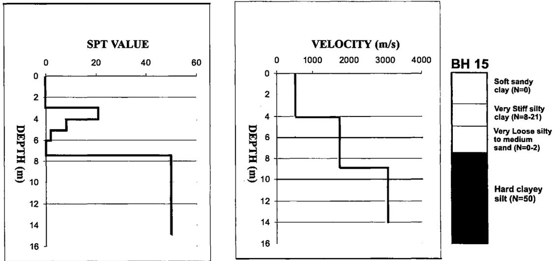
**Figure 3:** SPT values and 1-D velocity-depth curve for borehole 15
