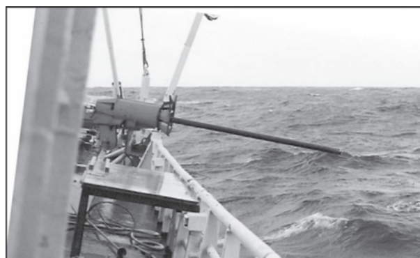
Figure 1. Special docking system for gravity coring.
