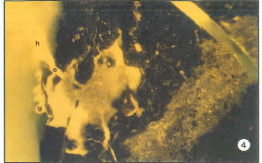
Figure 4. Generation of liquid hydrocarbons in the form of exsudatinite (e), oil globules (g) and oil haze (h) from bitumen. Note that bitumen, which originally fluoresces dull brown, increases its fluorescence intensity to bright yellow as a consequence of hydrocarbon generation: blue light excitation; field width = 0.26 mm.
