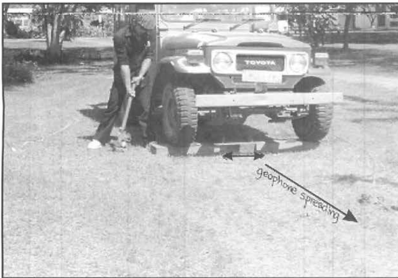
Figure 5. Wooden Plank, weighted by a truck (Youngme, 1985).
