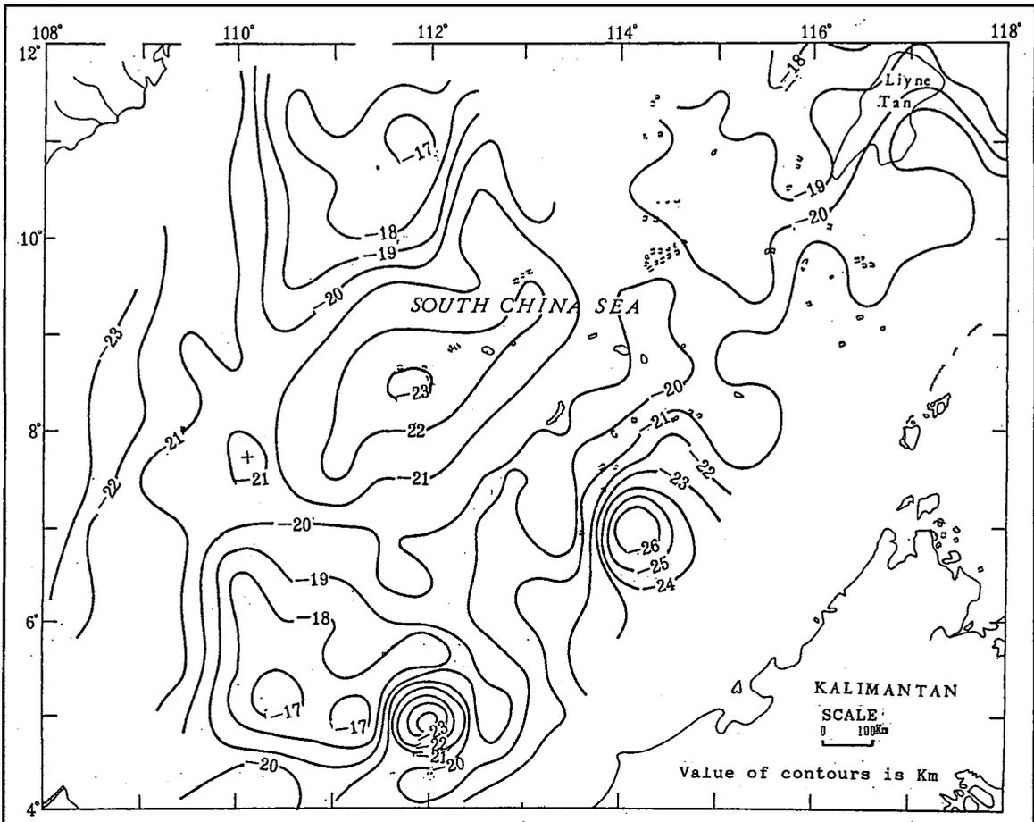
Figure 3. Depth map of the lower surface of magnetic body.
