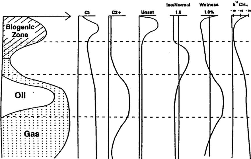
Figure 4: Hydrocarbon generation
