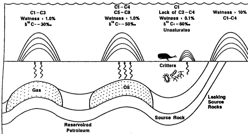
**Figure 3:** Primary sources of hydrocarbon seeps.
