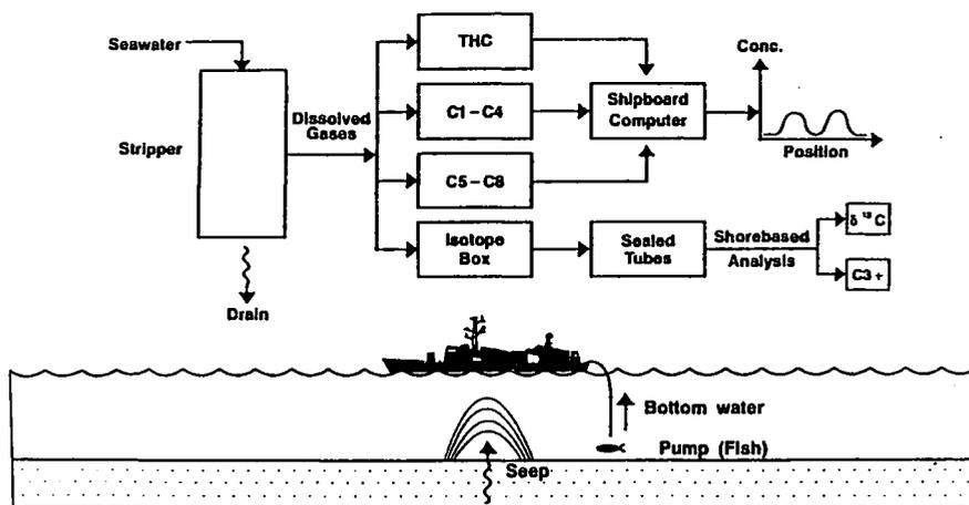
Figure 2: SNIFFER geochemical exploration method.
