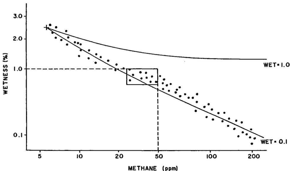
Figure 7: Plot of SNIFFER data from a location with high background wetness.
