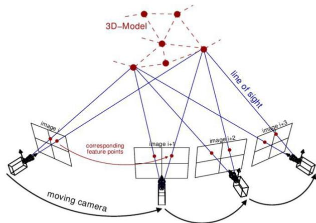
**Figure 2:** The illustration of photogrammetry method to create a 3-D model of an object from several images at different angles.
