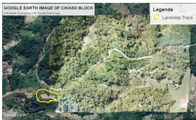
**Figure 6:** Overlapping photogrammetry image and Google Earth image has revealed the trace of an old landslide around the area of interest.
