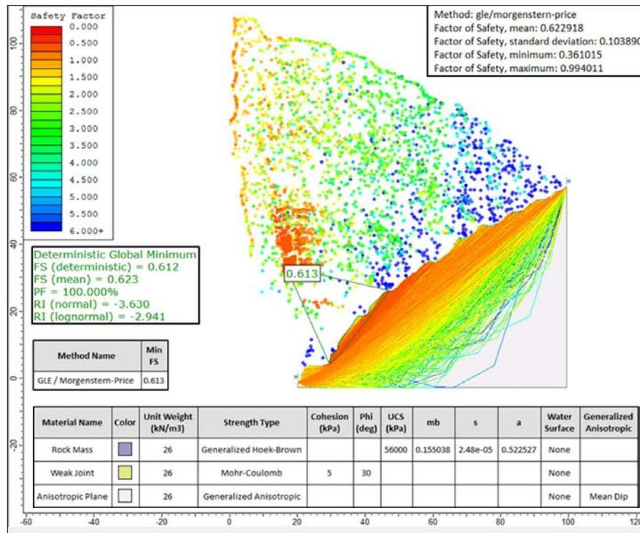
Figure 5: FoS of cut section with anisotropic plane in 2D.
