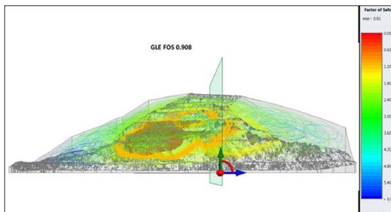
Figure 4: FoS of rock slope with anisotropic plane in 3D.
