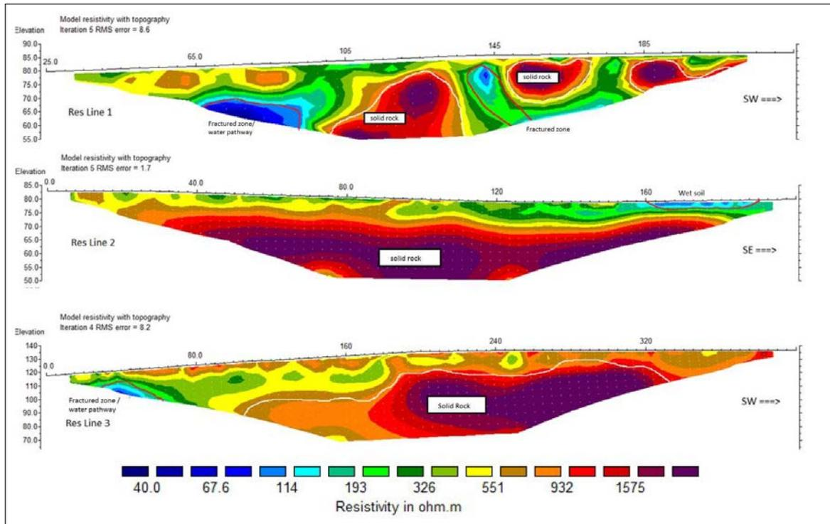
Figure 5: Geoelectrical resistivity model of line Res L1, Res L2 and Res L3.
