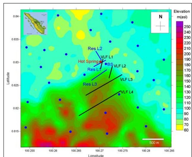
**Figure 2:** Topography map and location of the magnetic survey (blue circle), resistivity survey (blue line) and VLF survey (black line).
