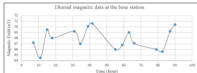
**Figure 3:** Diurnal magnetic data at the base station observed from 7:00 a.m. on the first day.
