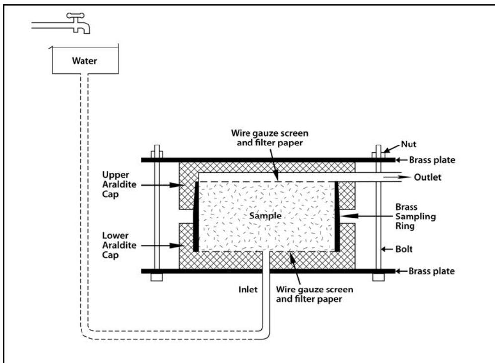
Figure 3: Schematic sketch of set-up for constant head permeability test.
