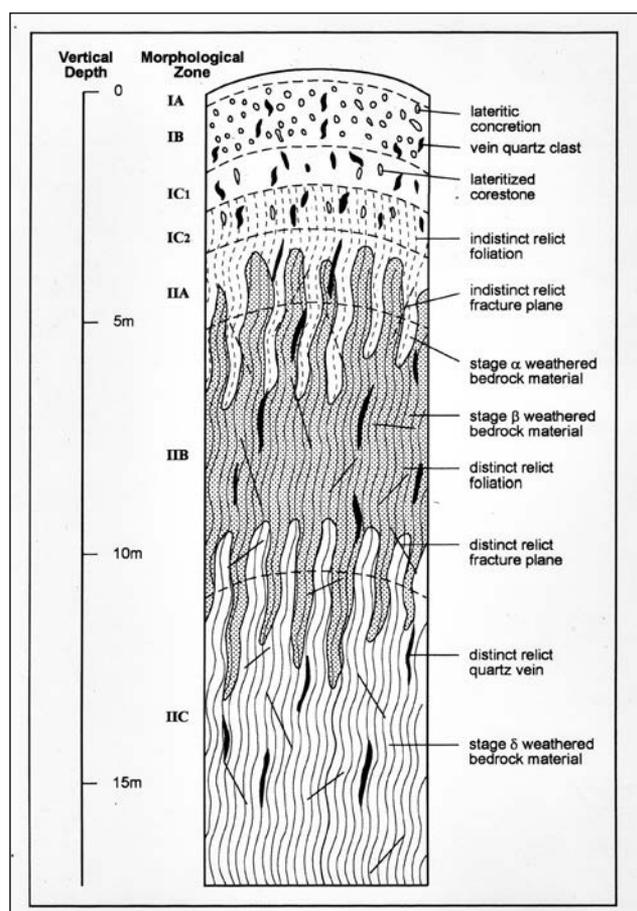
**Figure 2:** Schematic sketch of morphological features in the study site's weathering profile.
