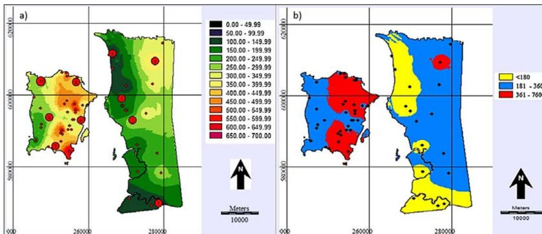
**Figure 2:** a)  $V_{s30}$  distribution map b) Soil profile classes based on NEHRP (Tan *et al.*, 2014).
