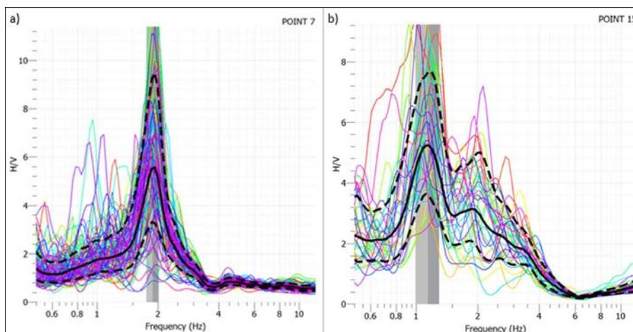
**Figure 6:** HVSR curves example generated from acquisition in Balik Pulau. a) Single clear peak at Point 7 b) Multiple curves at Point 15.
