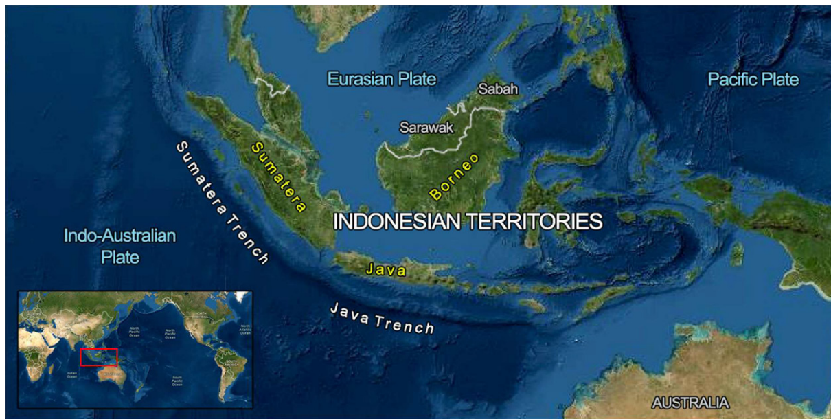
Figure 1: A topographic map of Indonesia with ocean bathymetry surroundings, illustrating Indonesian territories at the triple junction of the three major plates. Sumatra Trench and Java Trench are part of the Sunda Arc. Insert shows the position of the Indonesian archipelago (red rectangle) with respect to the globe. This is made available using ArcGIS Online Basemaps at https://arcgis.com/home/group.html accessed at 23/8/21.
