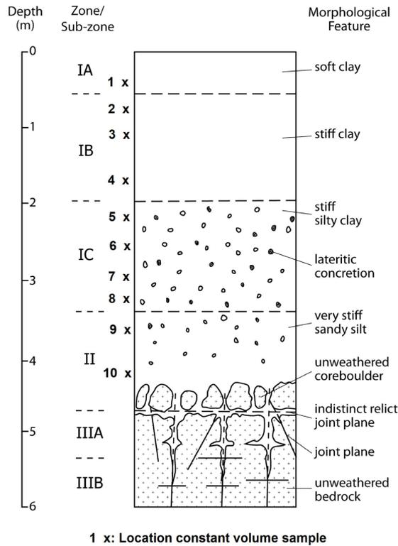
**Figure 2:** Schematic sketch of morphological features in the weathering profile with locations of constant volume samples (1 to 10).
