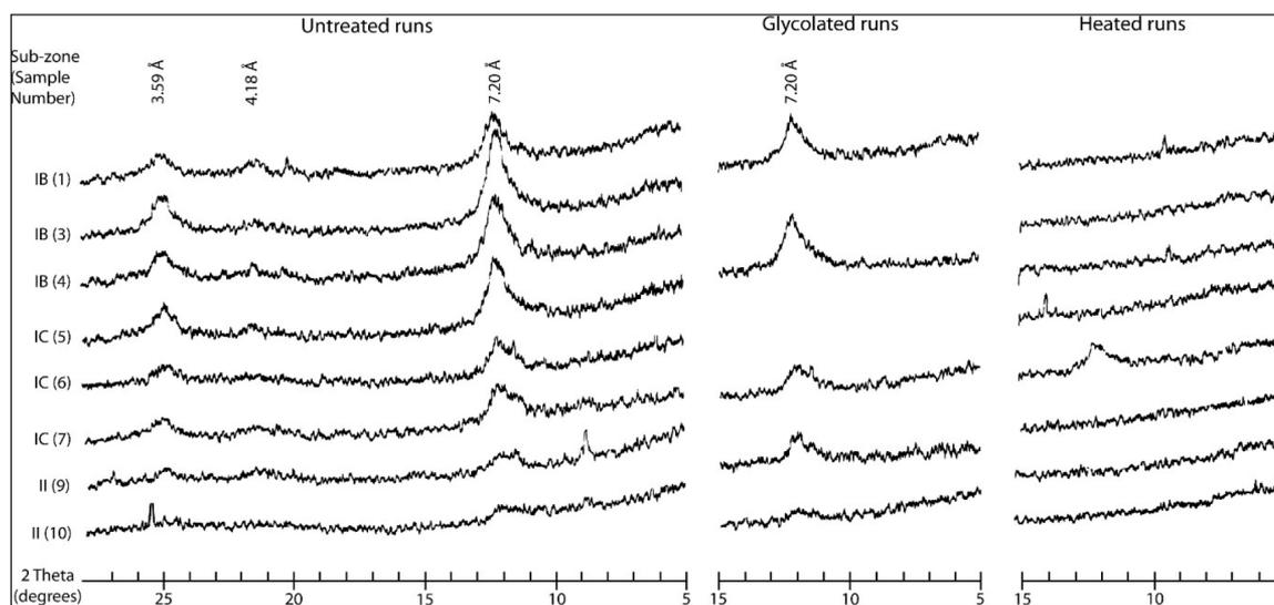
Figure 4: X-ray diffractograms of clay sized fractions in the weathering profile.
