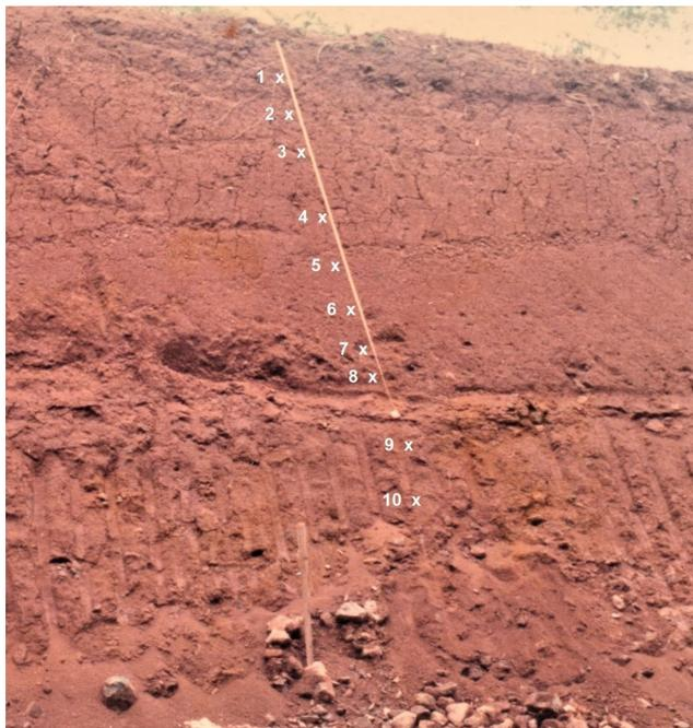
**Figure 3:** View of exposed weathering profile with locations of constant volume samples (1 to 10). (Tape is 3.90 m in length).
