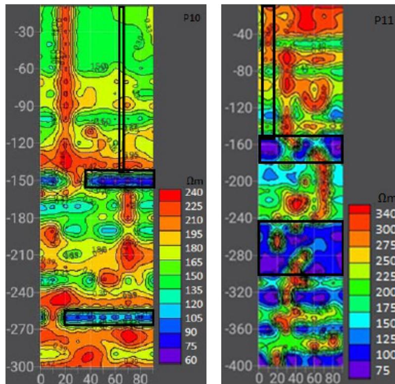
Figure 10: Electrical resistivity tomography of profile P10 and P11.
