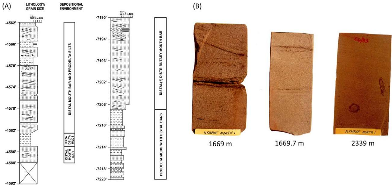
**Figure 16:** Core logs and examples of lithofacies in cores from Nymphe-1 North well (Barr, 1991). (A) Core logs of distal mouthbar and prodelta facies. Vertical scale in feet. (B) Examples of reservoir facies comprising medium and fine-grained sandstones.
