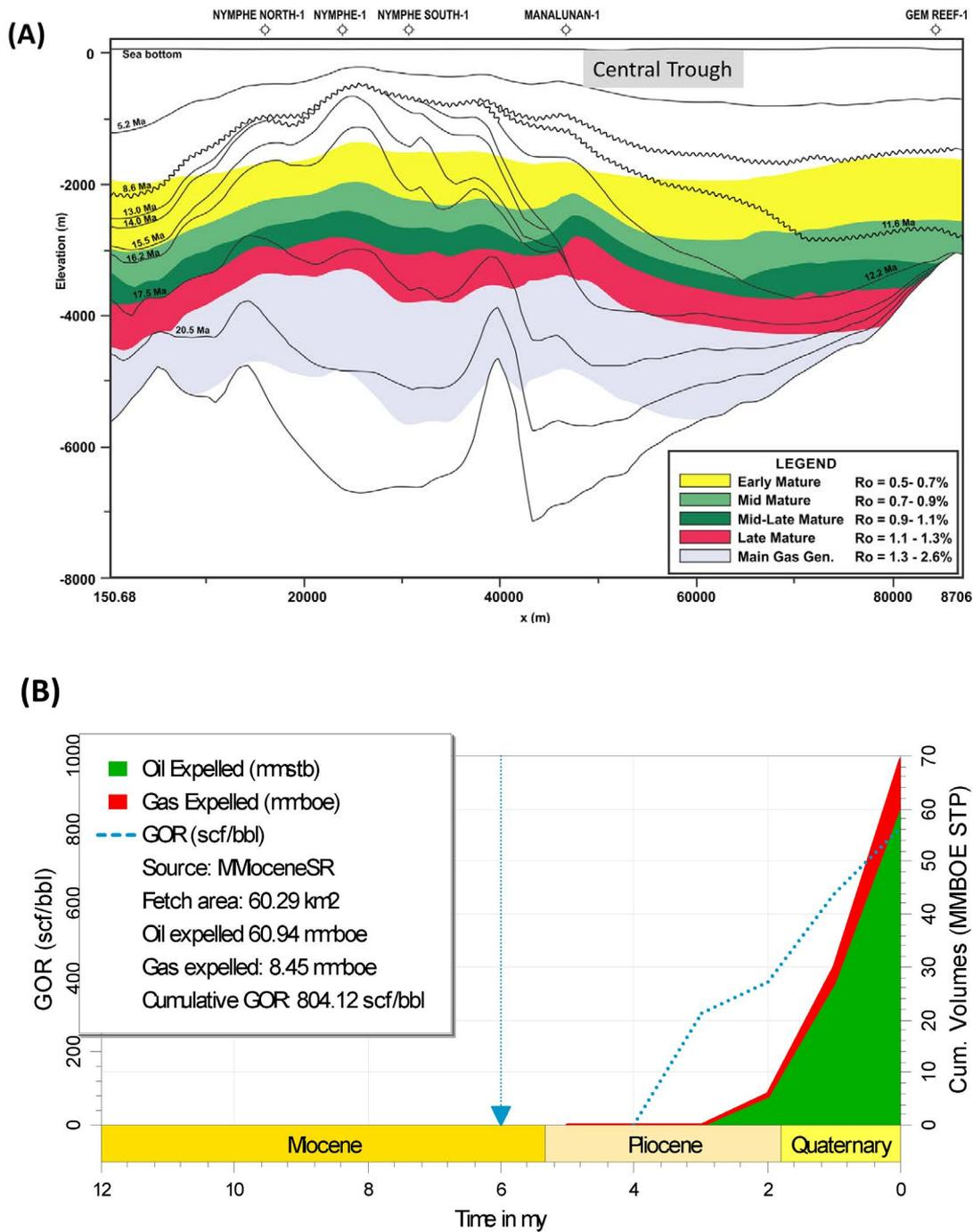
**Figure 19:** (A) Present-day maturity profile across the Sandakan Basin, along the Profile AA' (location in Figure 1). (B) Hydrocarbon expulsion model for the Sandakan Basin suggests that expulsion occurs mainly within the last 3 Myr (Mid-Pliocene) to present-day.
