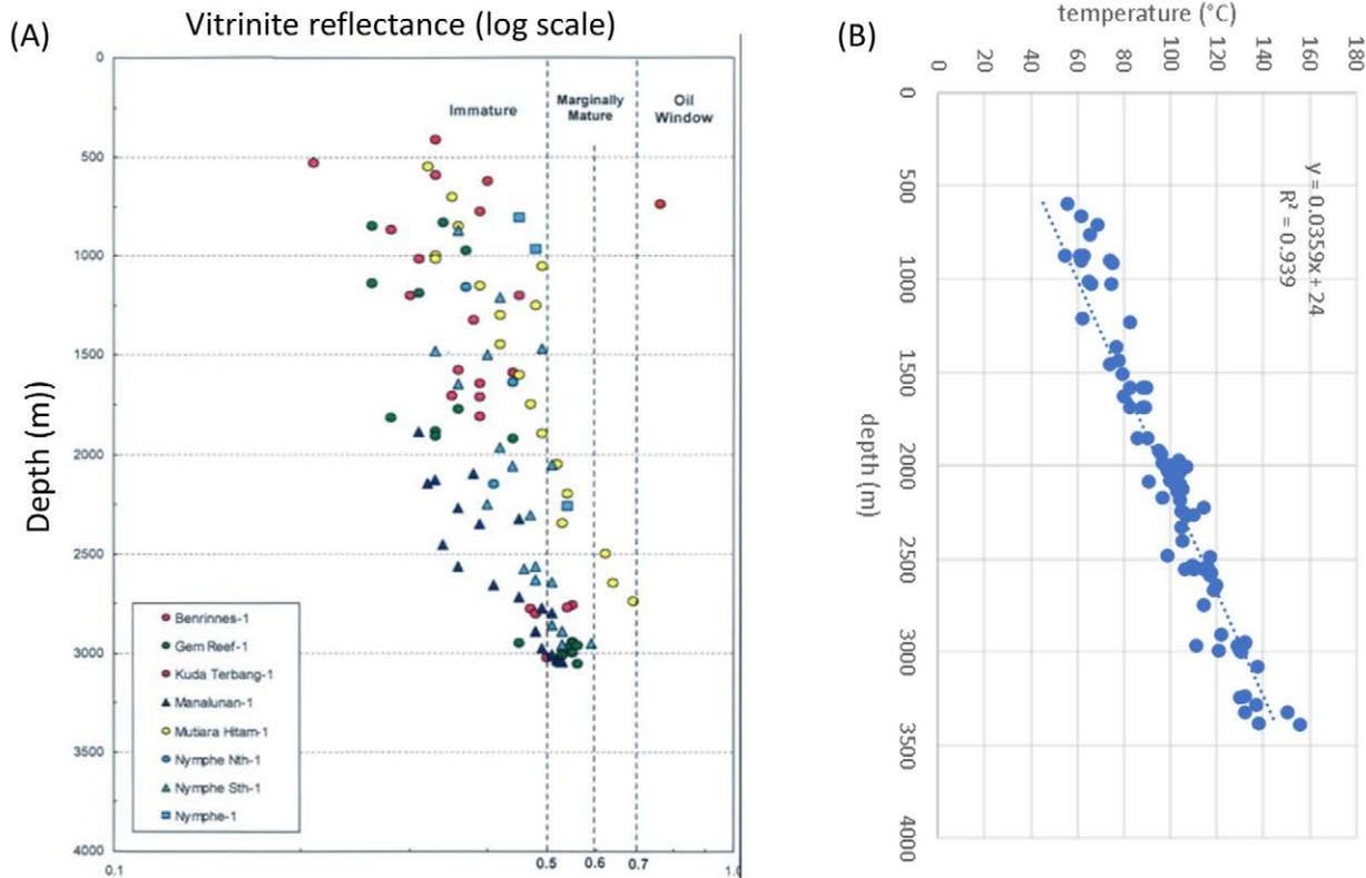
**Figure 18:** (A) Mean vitrinite reflectance ( $R_o$ ) vs depth in wells of Sandakan Basin. The data indicate that the penetrated section is currently in the early mature stage. (B) Corrected bottom-hole temperature (BHT) data, with regression line indicating average temperature gradient of  $35.9\text{ }^\circ\text{C}/\text{km}$ , assuming temperature at seabed of  $24\text{ }^\circ\text{C}$ .
