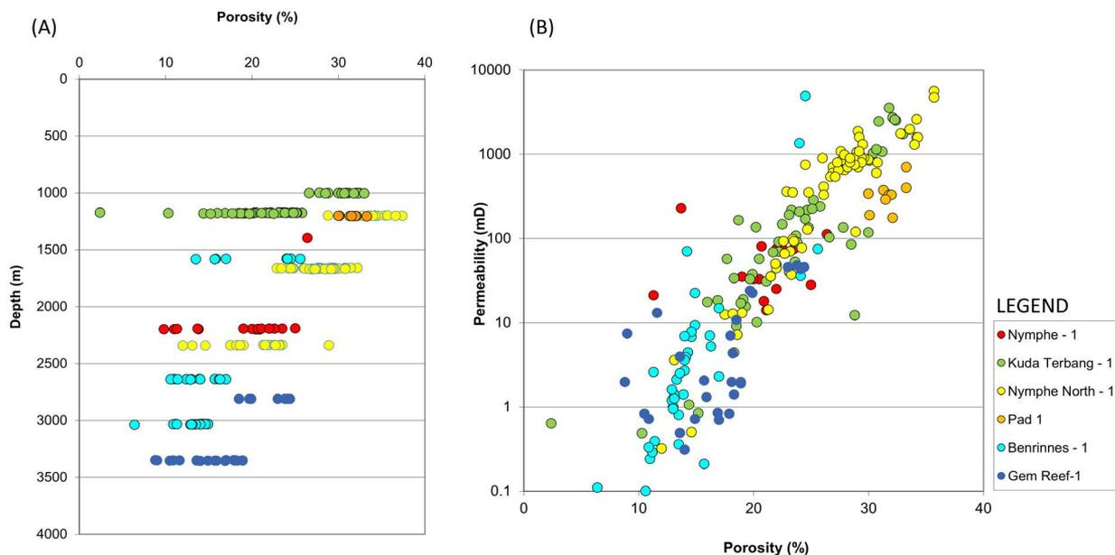
**Figure 17:** Porosity and permeability measured in cores from the Sandakan Basin. (A) Porosity and depth plot. Based on this dataset the porosity is expected to be less than 20% at ~3000 m, (B) Porosity-permeability relationship. At 3000 m, the permeability would generally be less than 10 mD.
