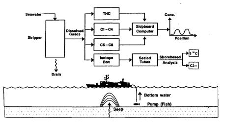
Figure 2: SNIFFER geochemical exploration method.
