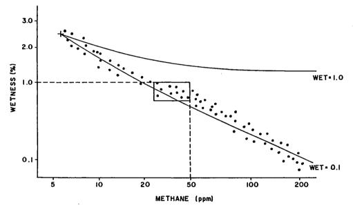
Figure 7: Plot of SNIFFER data from a location with high background wetness.
