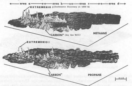
Figure 12: Methane and propane concentrations, northern Gulf of California.
