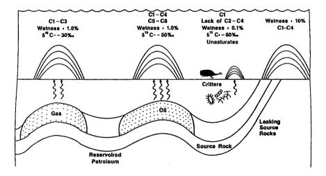
Figure 3: Primary sources of hydrocarbon seeps.
