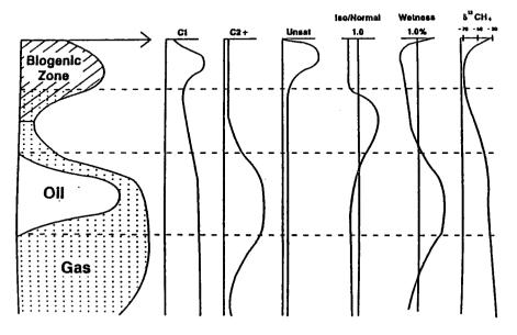
Figure 4: Hydrocarbon generation
