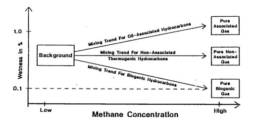
Figure 5: Seep characterization based upon mixing model.
