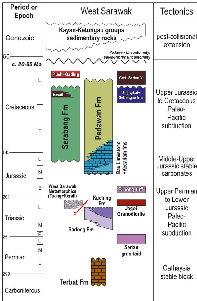
**Figure 3:** Pre-Cenozoic stratigraphy chart of West Sarawak (based on Liechti *et al.*, 1960; Hutchison, 2005; Breitfeld *et al.*, 2017). Note that the Kuching Formation is the deep-water lateral equivalent of the Sadong Formation. (V. – Volcanics; Fm – Formation; fms – formations).
