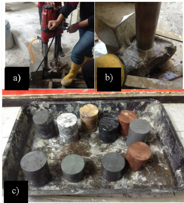
Figure 6: Cutting the rock sample into cylindrical shapes. a) the sample is placed in a jig specifically designed to hold the sample in place for both the trimming and facing, b) trimming the sample and c) cylindrical blocks.
