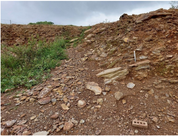
Figure 5: Recent excavation in overburden dump (25.03.2023) - Dumping 1937-1945 with coal extraction at Open-Cast No. 8 in Upper Coal Seam. (30 cm ruler for scale)
