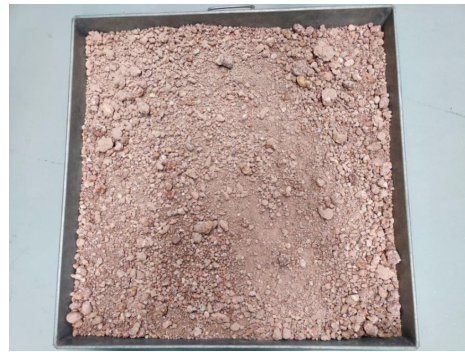
Figure 3: The soil-rock mixture collected from Segari Hill, Lumut is dried before sieving.
