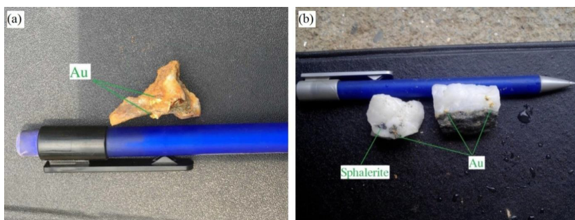
Figure 5: (a) Native gold and a symbiotic combination of quartz-arsenopyrite and pyrite, representing the first stage of mineral formation, and (b) Gold-quartz-polymetallic sulfide ore, characteristic of the second stage of mineral formation.
