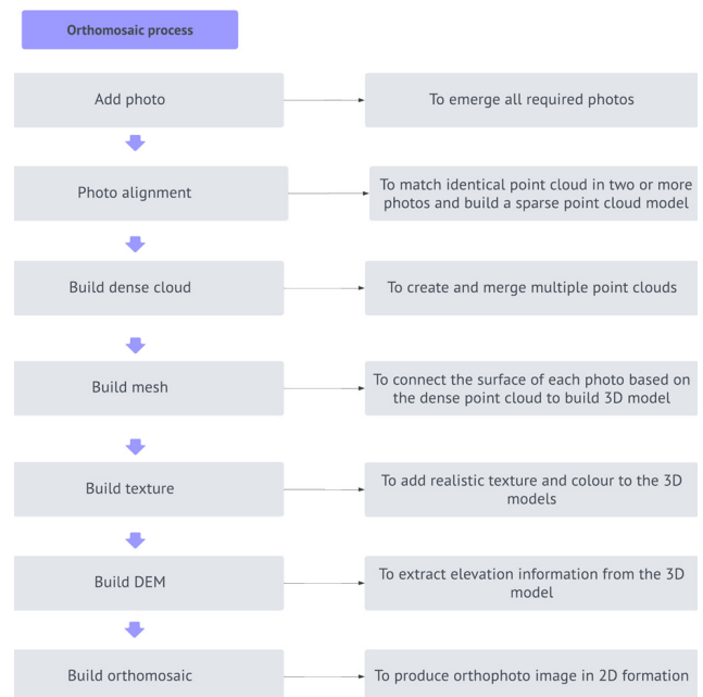
Figure 3: Process flowchart for orthomosaic creation in Agisoft Metashape.
