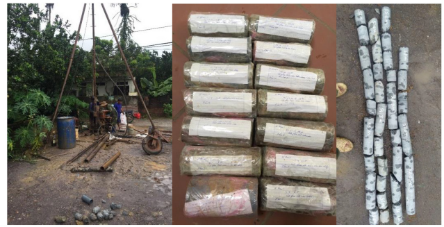
Figure 6: Well-bore geological survey, karst cave identification, and sampling.
