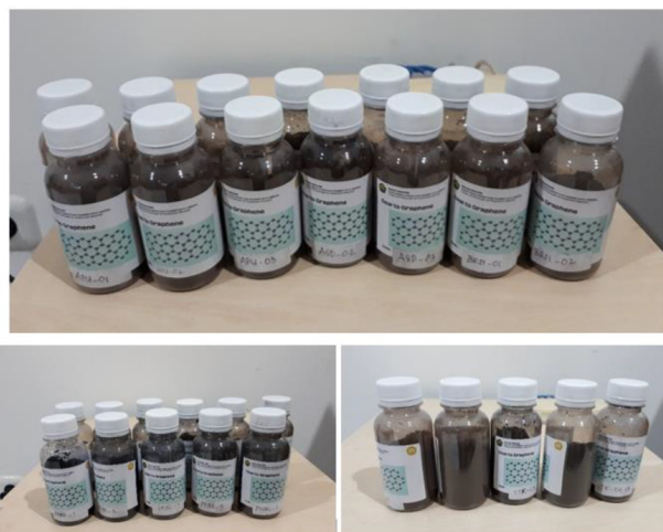
Figure 3: Graphene extracted from coal; graphene from Musi Banyuasin coal samples (top), graphene from Muara Enim and Lahat coal samples (bottom left) and graphene from East Kotawaringin coal samples (bottom right)
