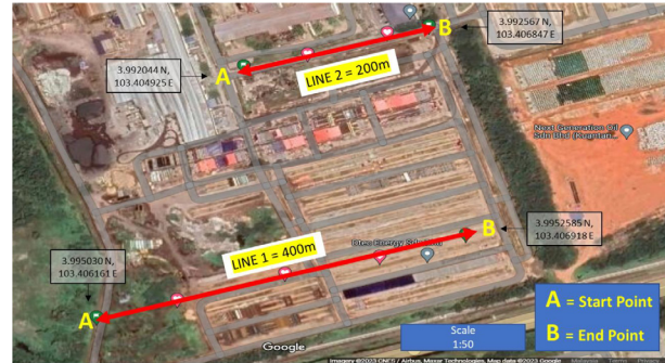
Figure 4: Actual survey line conducted at study area.
