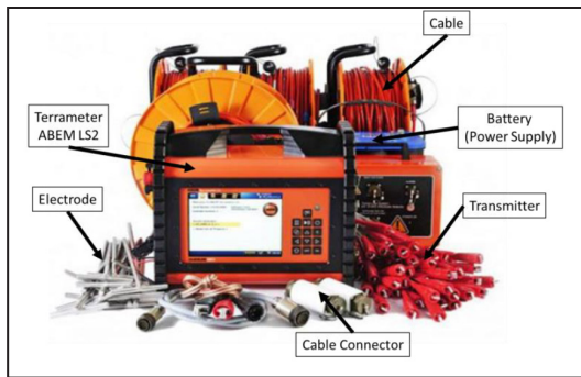
Figure 2: Multi-electrode resistivity meter system. Modified from Meterland (2024).
