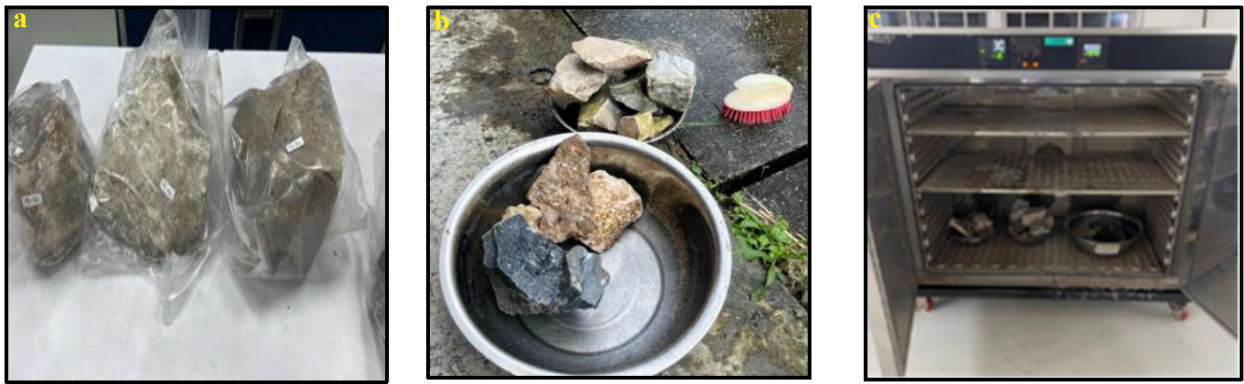
Figure 4: The laboratory procedures in preparing the samples for characterising tests (a) limestone samples, (b) washing process and (c) drying process in the oven.
