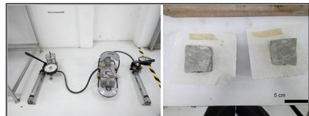
Figure 4: (a) Rock shear box apparatus (b) Sample in a mould for shear box testing.
