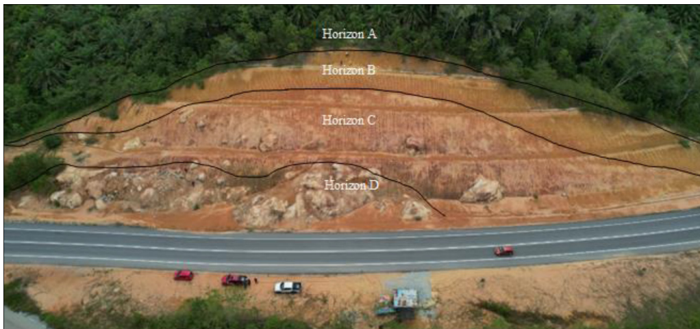
Figure 2: Exposed weathered granite profiles together with the bedrock at PUK site showing all the horizons.
