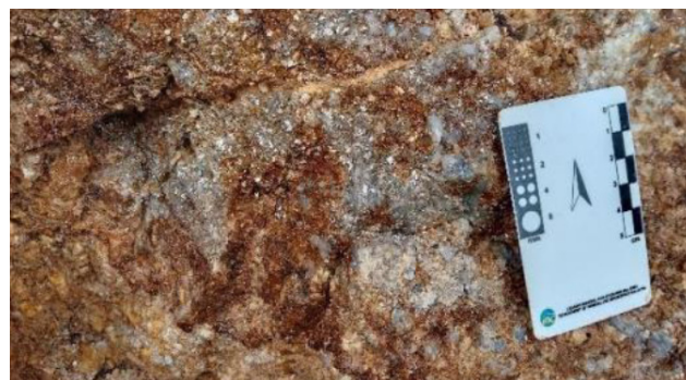
Figure 4: Altered (greisenized) granite with appearance of sericites found at northeastern part of Kampung Bandar (Kedah).
