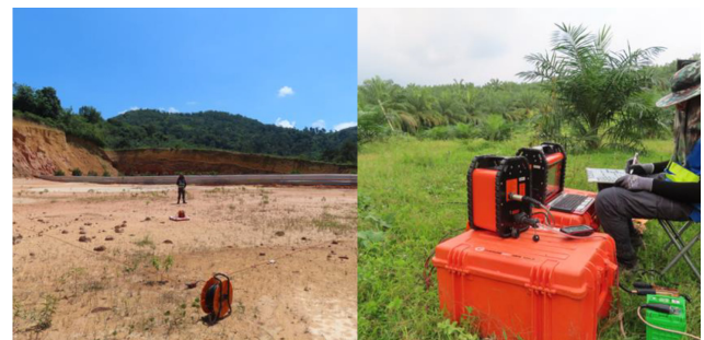
Figure 4: TEM survey conducted to identify the potential wellfields. The layout of the cables during the survey is shown on the left, while the right shows the TEM equipment, ABEM WalkTEM-2, used during the survey.
