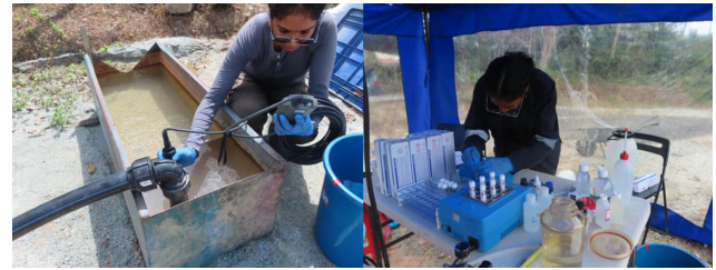
Figure 9: In-situ and on-site water quality analysis conducted during constant pumping tests, measuring the physical and chemical parameters.
