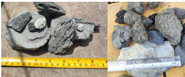
Figure 13: The large rock fragments flushed out during drilling at TW07.
