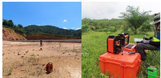
Figure 4: TEM survey conducted to identify the potential wellfields. The layout of the cables during the survey is shown on the left, while the right shows the TEM equipment, ABEM WalkTEM-2, used during the survey.
