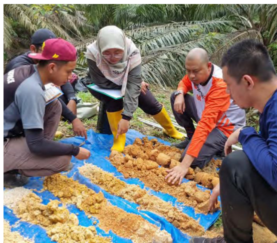
Figure 4: Soil samples arranged by depth for visual inspection. Observations include color determination using the Munsell soil color chart and identification of mineral grains.
