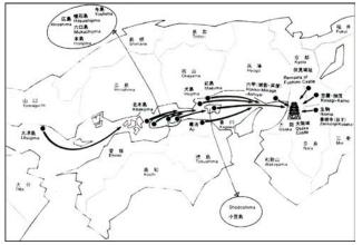
Figure 1: Origin of the granite used to construct the stone walls of Osaka Castle.
