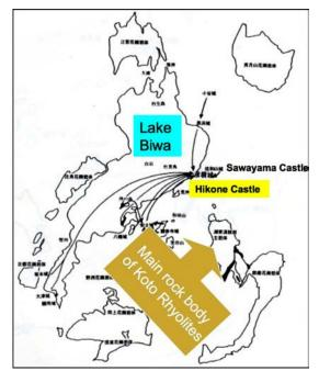
Figure 6: Origin of stones used in Hikone Castle. Many structures such as main keep, towers etc. were taken from other nearby castle because it was necessary to complete the castle as soon as possible in order to monitor the Toyotomi faction after the Battle of Sekigahara. The Hikone Castle stone was taken from the Late Cretaceous-Palaeogene Koto Rhyolite.
