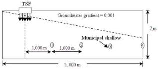
**Figure 2:** Schematic of the heavy metals transport leached from TSF through lateritic aquifer and positions of the assumed well nos 1-4 with 1 km distance between each well.
