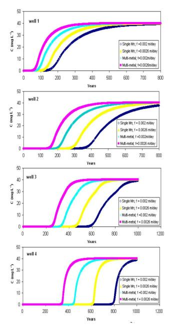
**Figure 3:** Concentrations of Mn<sup>2+</sup>in the lateritic aquifer under single metal, binary metal and multi-metal systems in four wells representing various distances from the contaminant source (see Figure 1).
