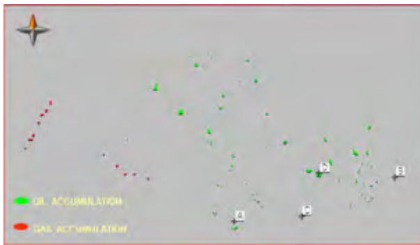
Figure 7: Representative modeling output showing hydrocarbon accumulation at Cycle II upper reservoir straddling MMU. Accumulation at discovery well location D in all the scenarios validates the study.
