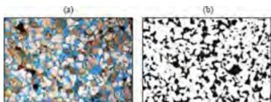
Fig. 1. (a) Scanned image from an epoxy-saturated thin section. Blue color denotes pores. (b) Binary image after image processing. The pore space appears in black.
