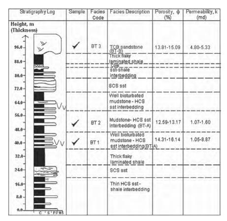
**Figure 5:** Sedimentological / stratigraphic log of the outcrop at Bintulu New Airport, in Bintulu, Sarawak.
