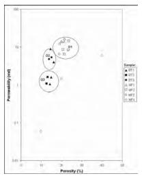
**Figure 6:** Permeability vs porosity crossplot for sandstone samples from Bintulu (Nyalau Formation) and Miri (Miri Formation), Sarawak.
