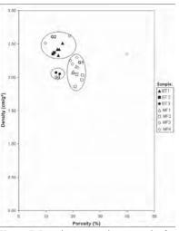
**Figure 7:** Density vs porosity cross-plot for sandstone samples from Bintulu (Nyalau Formation) and Miri (Miri Formation), Sarawak.
