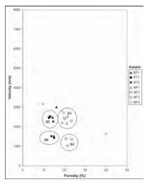
**Figure 8:** Velocity vs porosity crossplot for sandstone samples from Bintulu (Nyalau Formation) and Miri (Miri Formation), Sarawak.
