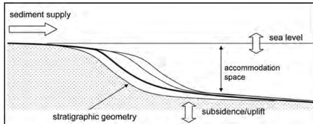
**Figure 1:** The main objective of stratigraphic simulation is to study the relative importance of the three primary factors controlling sequence development and stratigraphic geometries: sediment supply, subsidence/uplift, and sea-level change.
