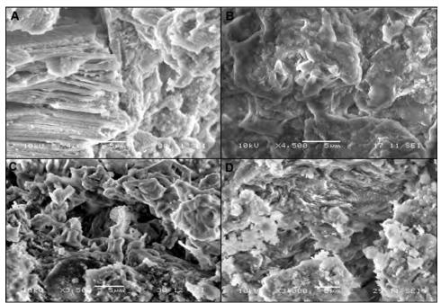
Figure 2: Scanning electron photomicrographs of volcanic soils showing (A) the layered of vermiculite minerals (B) subangular shapes of quartz minerals, (C) goethite in VS1 and (D) small dark spots showing the micropores within the layered structure of clay minerals.
