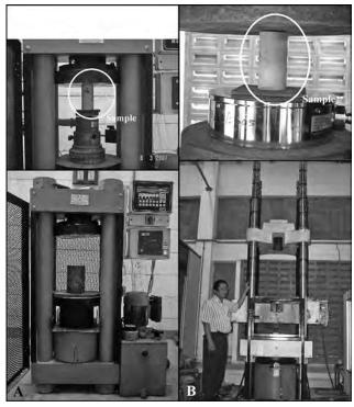
**Figure 5:** A) MaTest conventional compression testing machine prior to testing. B) Tinius Olsen servo-controlled testing machine prior to testing.
