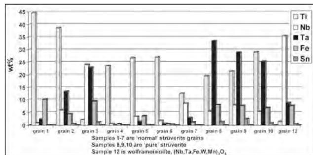
Figure 4: Chart showing variable contents of Ti, Nb, Ta and Fe in struverite concentrates.
