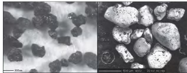
Figure 2: Under the binocular microscope (left), struverite is a greyish to dark grey, sometimes black mineral. EPMA BSE image (right) show struverite grains crystallizing in the tetragonal system and common habits are prismatic and bipyramidal tetragons. Scale bar is 0.3 mm.
