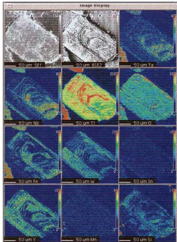
Figure 8: EPMA X-ray map of zoned strüverite showing the distribution of Ta, Nb, Ti, Fe, W, Sn, Mn and Y within zones in the grain. Sample BEH struv2.
