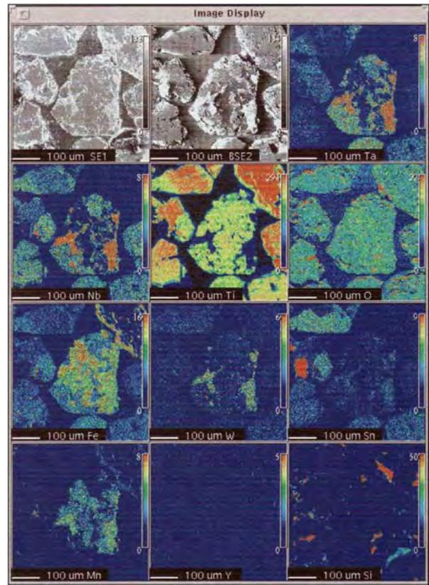
Figure 6: EPMA X-ray map of strüverite grain showing exsolved bodies rich in Ta, Nb, Ti, Sn, Mn and Fe with a rim of ilmenite ( $\text{FeTiO}_3$ ). Sample BEH10.
