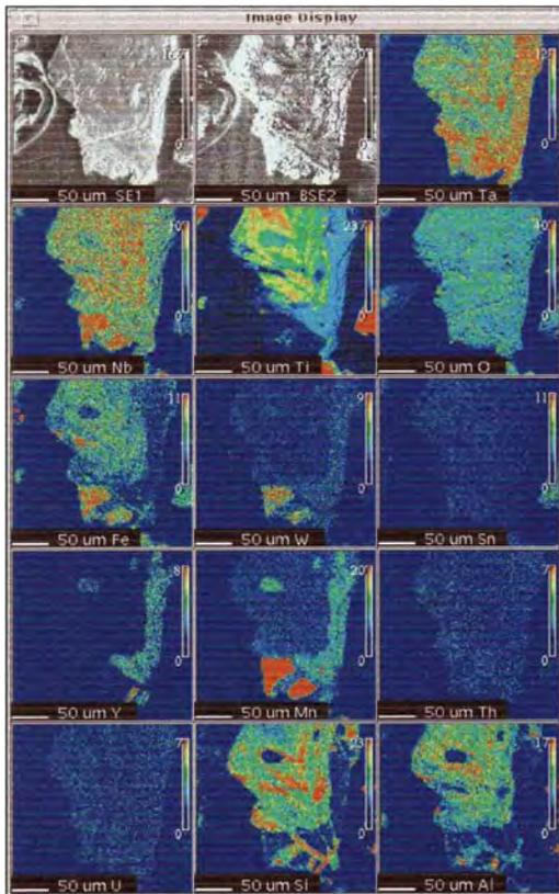
Figure 7: X-ray map showing strüverite grain with exsolved columbite ( $\text{Nb}_2\text{O}_5$ ), tantalite ( $\text{Ta}_2\text{O}_5$ ) and wolframioxiolite ( $\text{Ta,Nb,Fe,W,Mn}_3\text{O}_4$ ). Sample Bidor.
