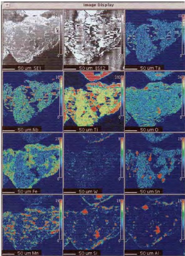
Figure 5: Chart showing the variation in Ti, Nb, Ta, Fe, and Sn contents of struverite grains.
