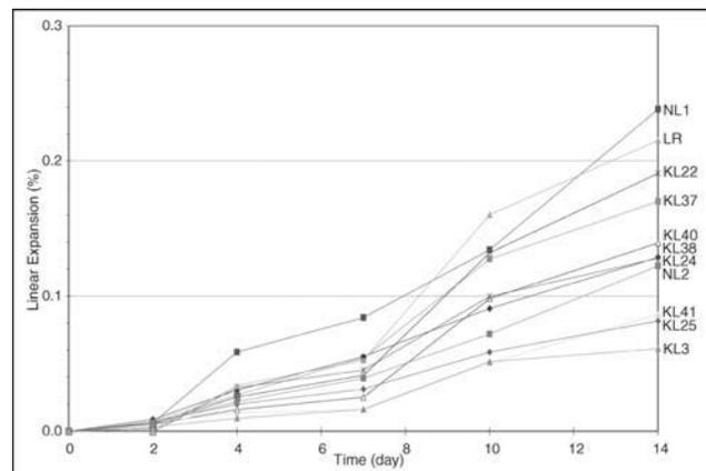
Figure 4: Results of the ASTM C1260 mortar-bar test. Linear expansion values are averaged from three bars, time is days of immersion in NaOH. Sample LR=Lanchang rhyolite.
