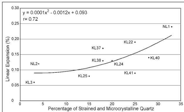
Figure 5. Plot of linear expansion of the mortar-bars against total strained and microcrystalline quartz content.
