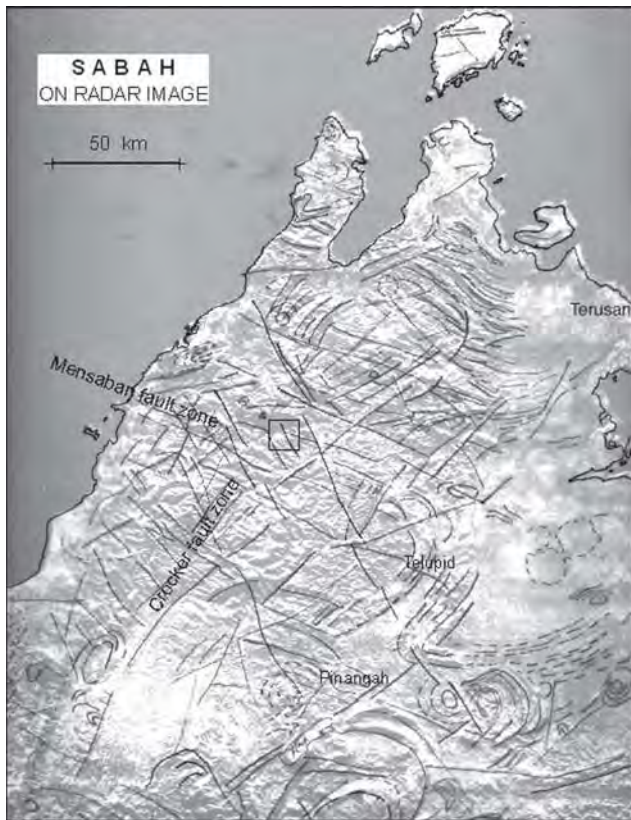
Figure 1: Lineaments and curvi-lineaments on radar image of western and central Sabah. Kudasang (square) lies at the intersection of the Mensaban and Crocker fault zones. In the east, the Mensaban fault zone terminates against a major tectonic lineament that extends from Terusan via Telupid to Pinangah. A large multi-ring structure south of Marudu Bay centres about Marak Parak and could represent an impact structure.
